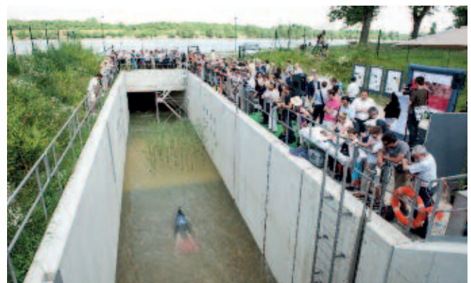
Figure 2. Experimental research channel at BOKU University, Vienna, being used for 1:1 scale sediment transport tests
