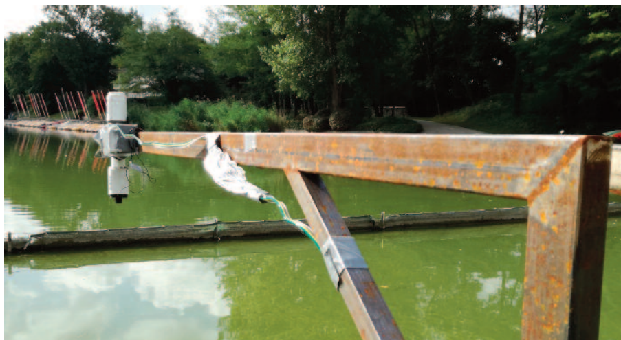
Figure 3. Optic sensor at a fix position at Champs sur Marne (Photo C. Freissinet)
