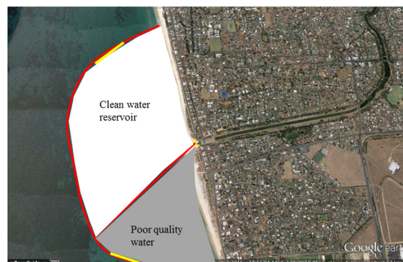
Figure 7. Coastal reservoir at Torrens River mouth, total length of its dike is 16 km, about 1/3 of its area is used for storage of poor quality water that can be used to feed the desalination plant or irrigation.
