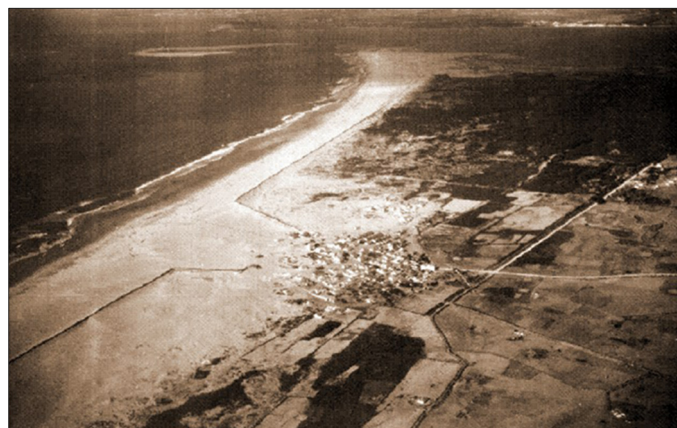
Figure 5. Old aerial photo of the small fishing village of Costa da Caparica (1937) protected by a long dyke built by the army after a flooding wave event.
