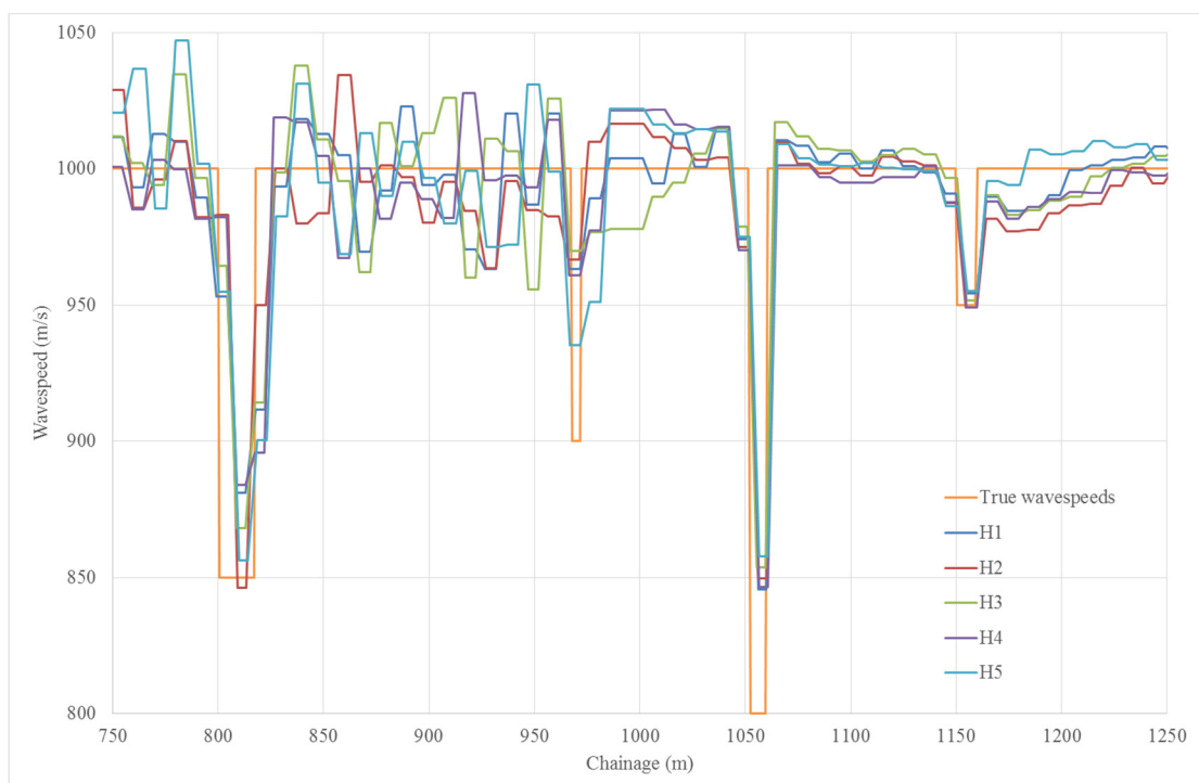
Figure 8. Wavespeeds estimated by ITA using different sets of pressure traces with high noise.
