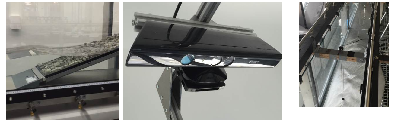
Figure 3. (Left) – Beached bed, (Centre) – Kinect mounted above flume, (Right) – Conductance wave probe.
