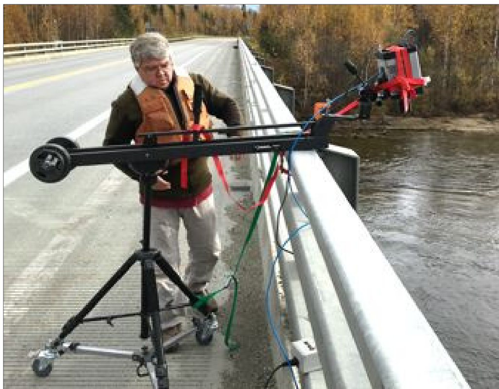
Figure 2. Photograph showing infrared camera positioned on a bridge over the Salcha River.
