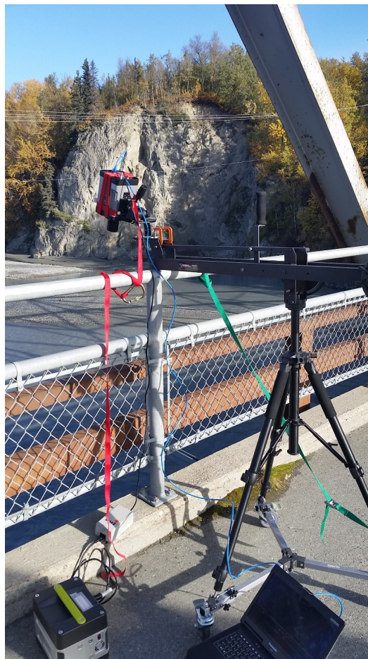
Figure 2. Picture of the deployment apparatus and the cooled, mid-wavelength infrared camera as deployed on the Matenuska River. All the Alaskan sites used the same arrangement for stationary measurements.
