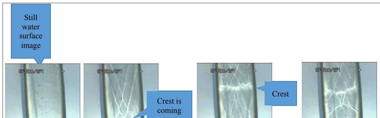
Figure 7. Recorded images of fringe patterns in brightness on the bottom of the channel.
