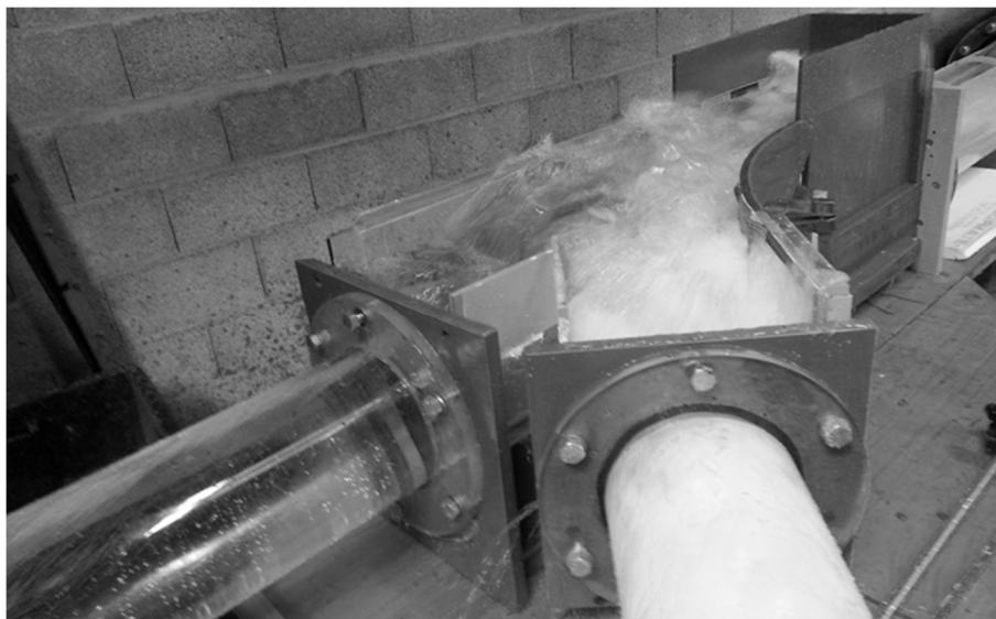
Figure 3. Choking of the junction manhole due to the abrupt pressurization of upstream branches, as observed in 45^\circ junction manhole with bottom drops under set-up E (see Table 1).
