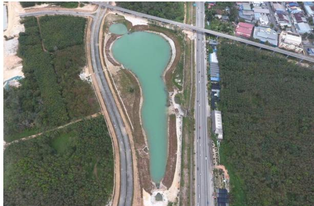
**Figure 9.** Detention pond with sediment forebay.
