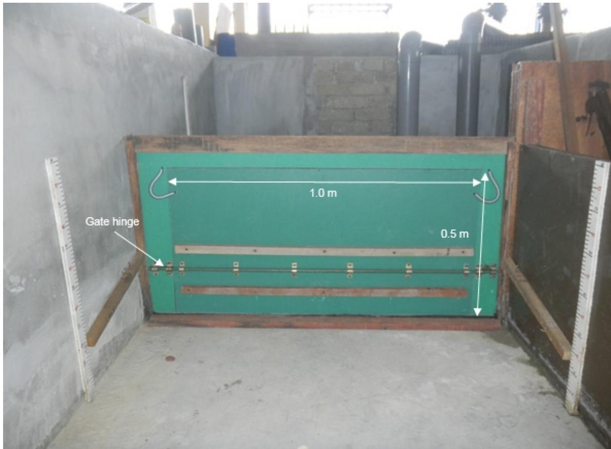
Figure 1. Front view of the tipping flush gate.
