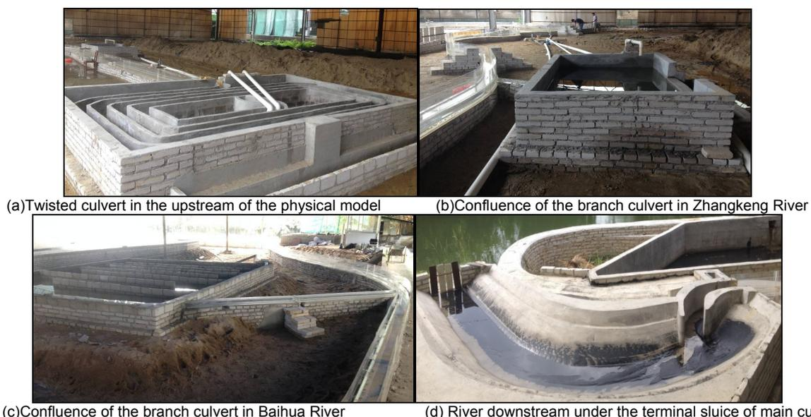
**Figure 7.** The boundary simulation photos of physical model for long distance sewage interception culvert.
