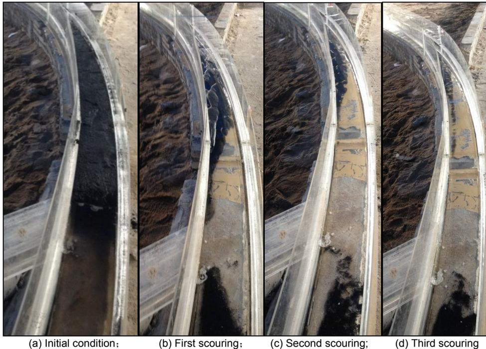
**Figure 11.** Terrain in sewage culvert after the third scouring test at Baihua River branch culvert (Z1+888).
