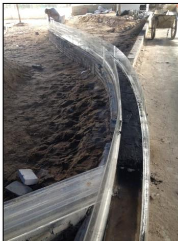
**Figure 8.** Initial condition for water storage and scouring test.
