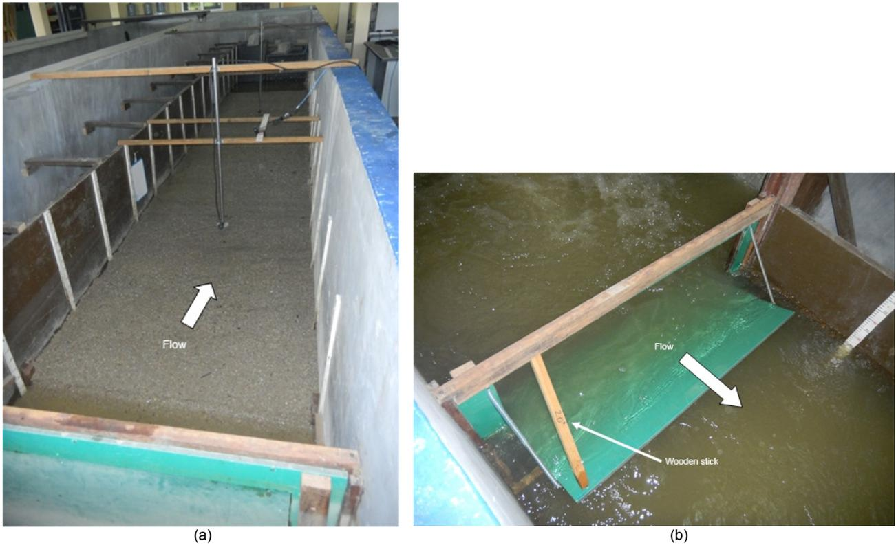
**Figure 3.** Experimental set up: (a) general view and installation set up for the flushing experiment; and (b) wooden stick to prevent the gate from closing after flushing for the 30 minutes and 60 minutes duration experiments.
