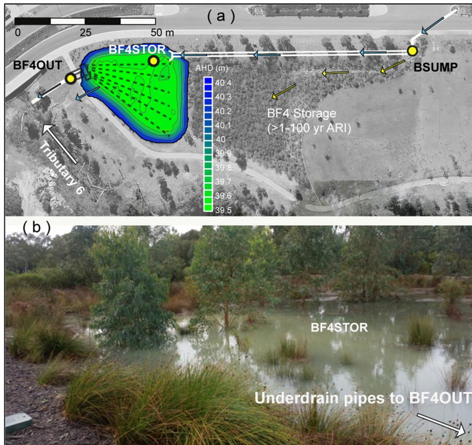
**Figure 2.** Bioretention basin drainage components and view: a) Bioretention basin (BF4) for the 1-yr ARI event, and b) view of the storage area (BF4STOR) after small rainfall event. Dashed lines in (a) represent underdrain slotted pipes. Elevation in contour map corresponds to Australian Height Datum (A.H.D.).
