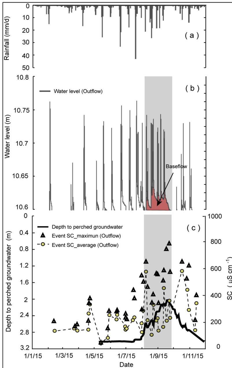
**Figure 3.** Hydrological and tracer data for selected events in 2015: a) rainfall total (mm/day), b) bioretention basin outflow hydrographs (BF4OUT), c) depth to perched groundwater and specific conductance (SC) corresponding to bioretention basin outflow. Depth to perched groundwater (m) from ground level. Shaded areas indicate time of groundwater interactions with the bioretention basin.
