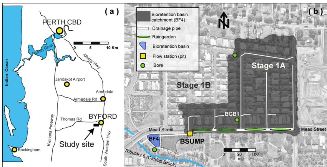
**Figure 1.** Study site area and bioretention basin location: a) Location of Byford area and b) The Glades Stage 1 (A and B) and bioretention basin (BF4) location on the treatment train.
