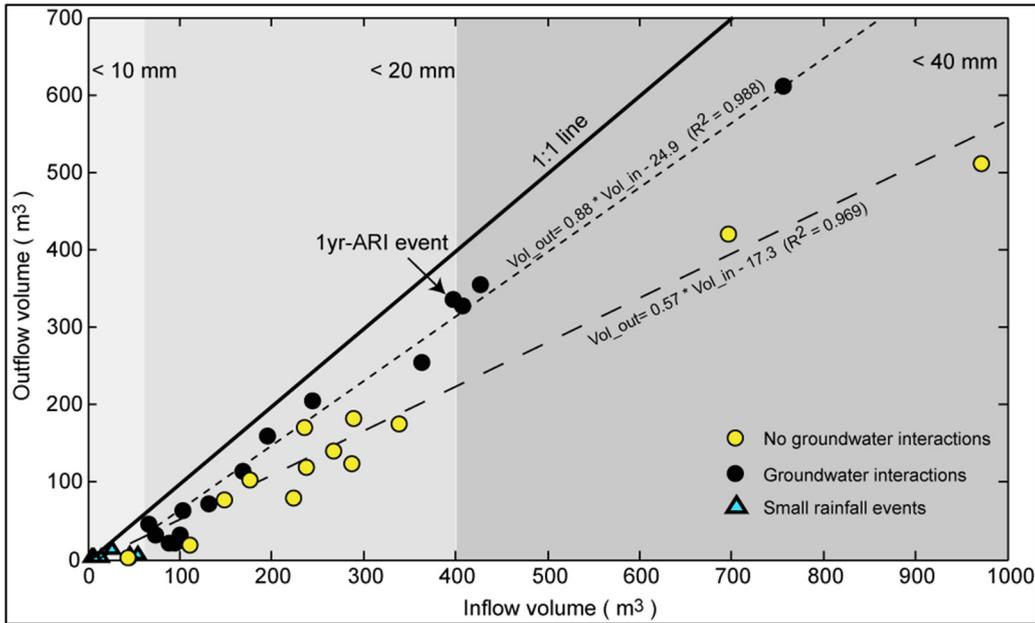
**Figure 4.** Volumetric performance of the bioretention basin for the 37 events. Shaded area indicates rainfall event magnitude. Regression lines and equations for both data sets are included.
