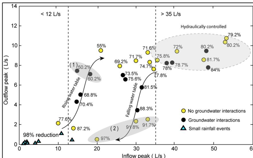
**Figure 5.** Peak flow reduction performance for all events. Light-grey shaded area indicates inflow peaks > 35 L/s and events with outflow controlled by surface water storage discharge from the basin. Dark-grey shaded area and numbers in brackets highlight events of similar characteristics showing performance differences in relation to groundwater dynamics (S-shaped lines).
