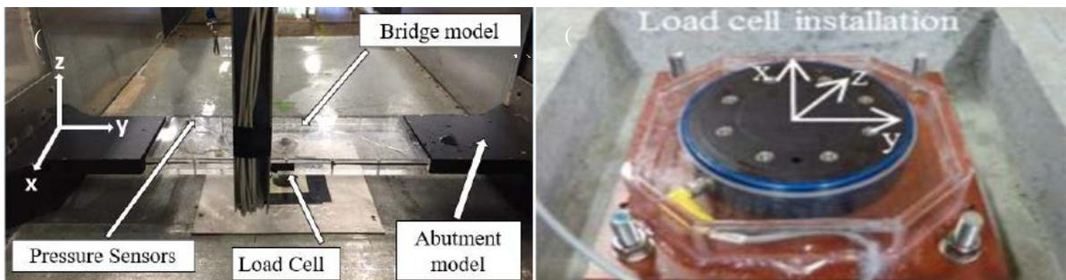
**Figure 6.** Pressure sensors and load cell installation.
