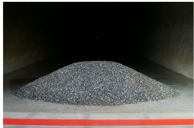
Figure 9. Input sediment ( D_s = 10 mm, V = 5 m 3 /s).
