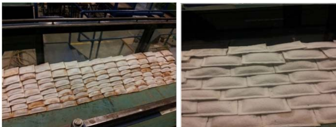
Figure 2: Revetment construction - stack bond (left), running bond (right)
